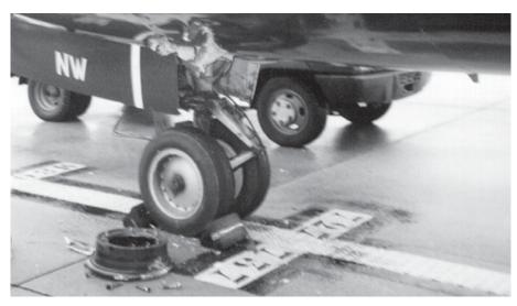
Split hub lying below the hole in the fuselage
